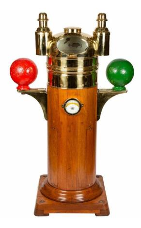
One of CMM's most colorful, eye-catching artifacts is a compass and navigational instrument housing station called a binnacle. The instrument was salvaged from the *S.S. Harvester*, a 525-foot all-steel, single screw propelled bulk carrier. Built-in Lorain, Ohio in 1911, the ship served on the Great Lakes until being scrapped in 1977.
